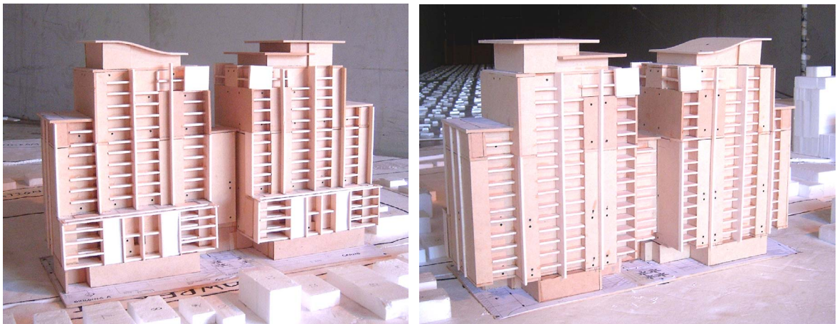
Figure 2: Photographs of the model in the wind tunnel
