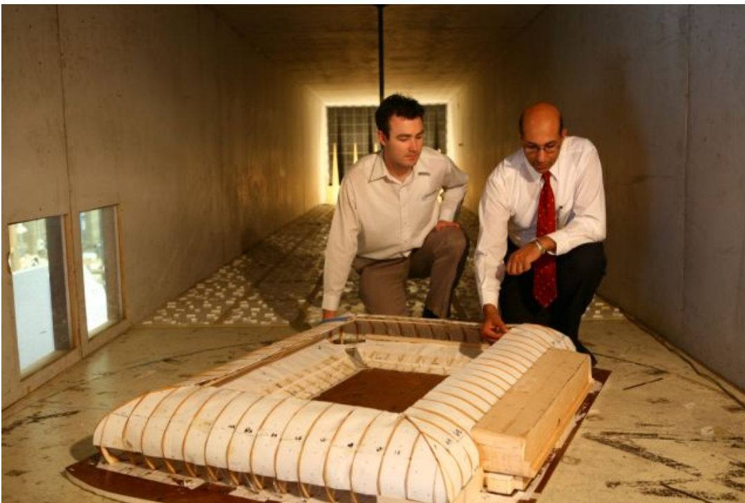
Figure 8. The 1:150 scale model of the Gold Coast Stadium in Windtech's Boundary Layer Wind Tunnel.
