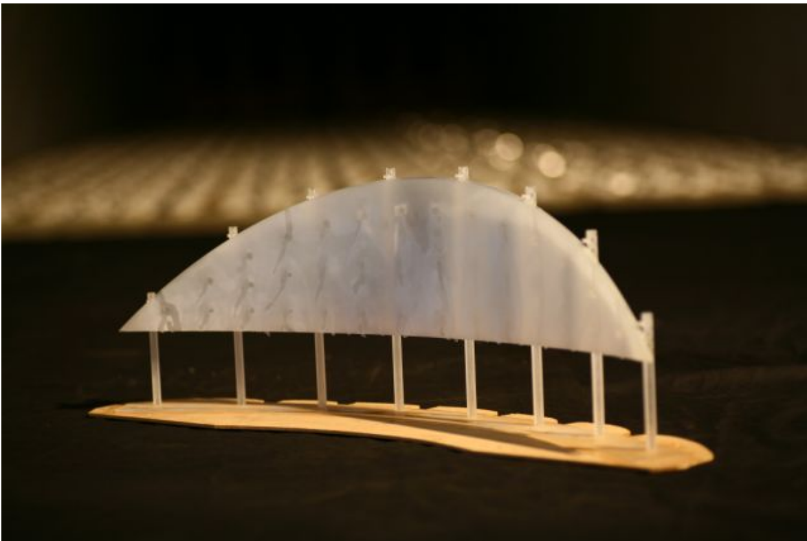
Figure 17. The 1:300 scale pressure-tapped impermeable model of the LED screen for the 2006 Asian Games, Doha.
