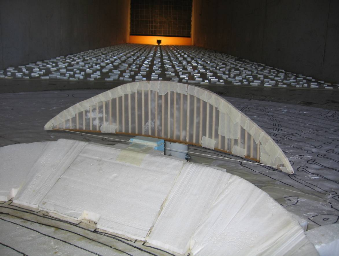
Figure 14. The 1:300 scale impermeable model of the LED screen for the 2006 Asian Games, Doha connected to the force balance.
