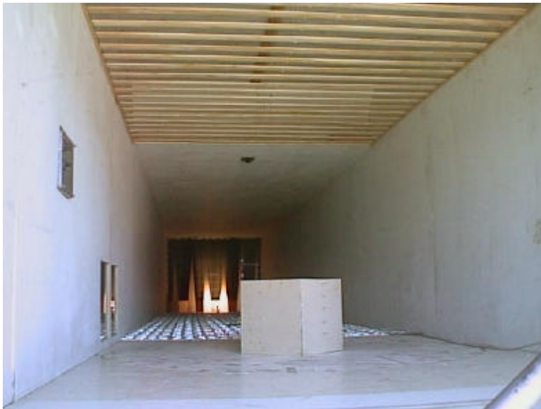
Figure 2: The 4.4% blockage cube in Windtech's blockage tolerant boundary layer wind tunnel, at incidence angle 45 degrees.
