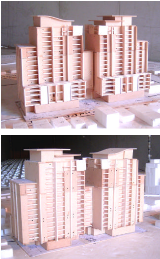
Figure 1: Photographs of the model in the wind tunnel
